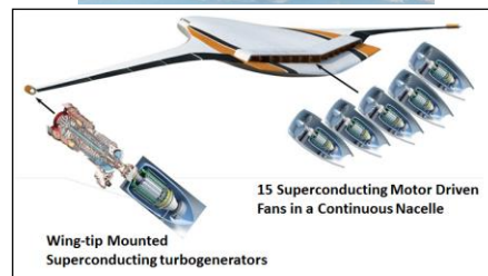
Figure 6. N3-X hybrid wing body (HWB) aircraft with a turboelectric distributed propulsion (TeDP) system [54].
