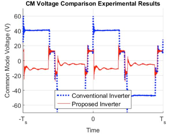
Fig. 5. Experimental measurements of CM voltage of a conventional sine PWM inverter and proposed inverter.
