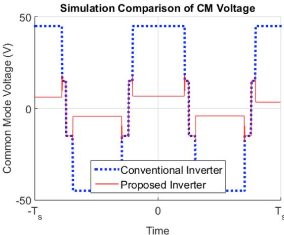
Fig. 3. Simulation of common mode voltage of conventional inverter compared to proposed inverter.
