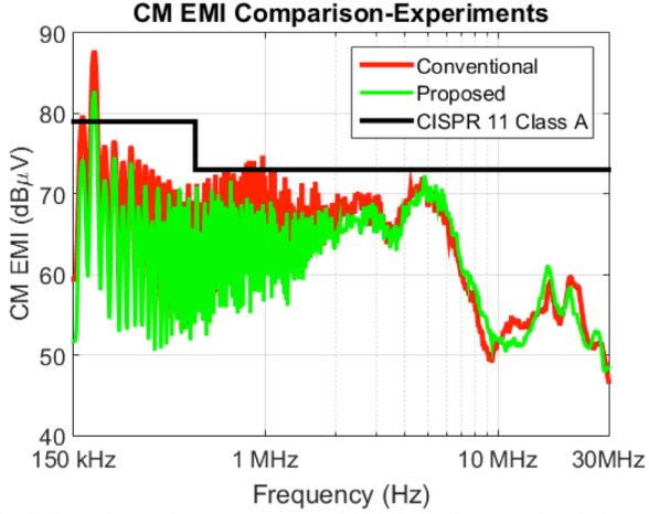
Fig. 7. Experimental measurements of CM EMI of conventional six switch sine PWM inverter and proposed inverter.
