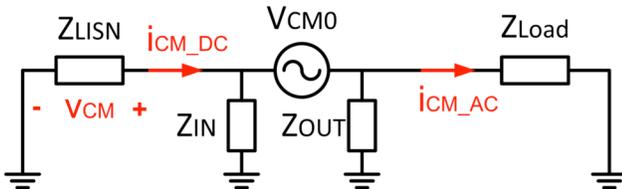
Fig. 8. Model of CM EMI noise coupling path. Both the conventional and proposed inverters have the same impedance values, with only the voltage source different.
