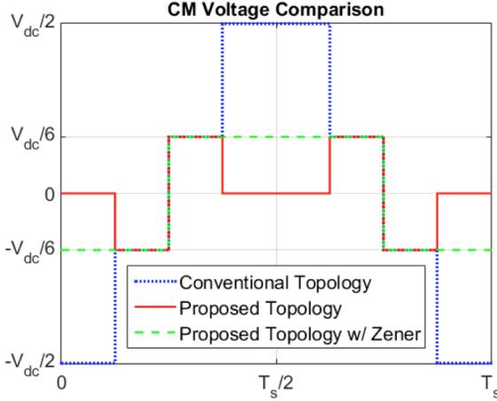
Fig. 2. Common mode voltage of conventional inverter compared to proposed inverter.
