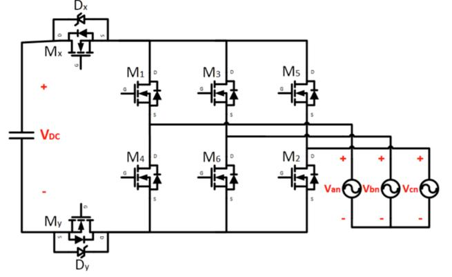
Fig. 1. Proposed inverter topology with extra switches between phase legs and DC capacitors.
