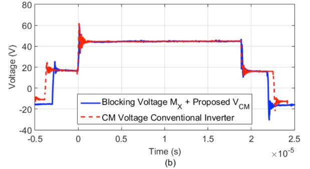
Fig. 6. (a) Blocking voltage of the proposed topology, blocking the DC bus during the zero state allowing for the reduction. (b) Sum of the blocking voltage and CM voltage of proposed inverter compared to conventional inverter CM voltage.
