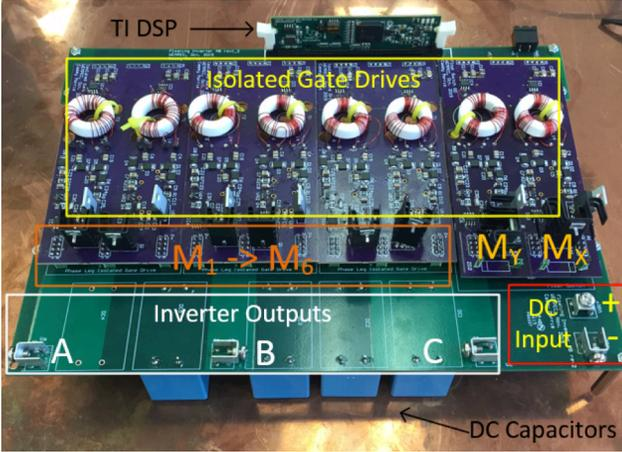
Fig. 4. Realization of the proposed inverter, created in a modular fashion, with key components labeled, photographed on top of copper ground plane.
